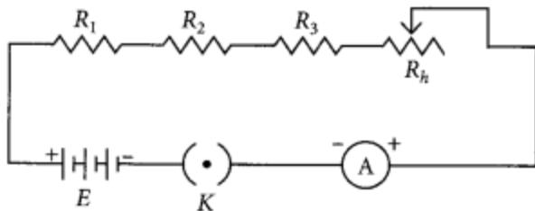
Change the positions of ammeter and note the reading of ammeter each time. You will find that all the reading obtained are same.
