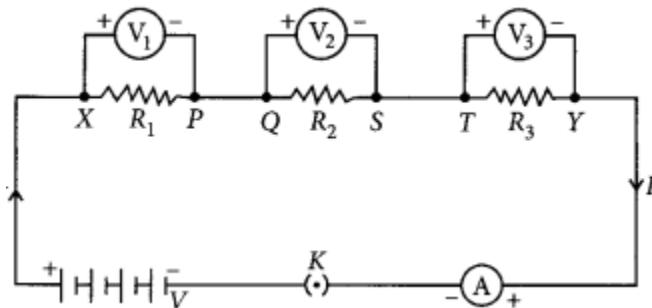
Given figure shows the series combination of three resistors  $R_1$ ,  $R_2$  and  $R_3$  connected across a voltage source of potential difference  $V$ .
