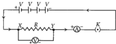
The shape of the graph obtained by plotting potential difference applied across conductor against the current flowing v. Ilmuigh il will be a straight line.
