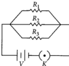
$$\frac{1}{R_{eq}} = \frac{1}{R_1} + \frac{1}{R_2} + \frac{1}{R_3}$$
